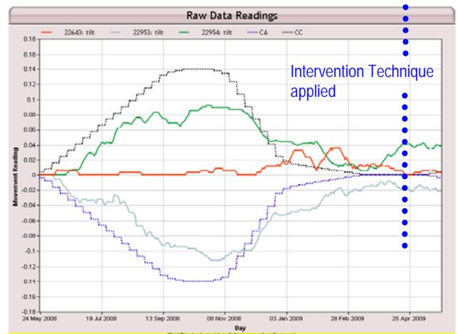
The underlying algorithm that "pattern matches" to arrive at a probability of the data being root induced clay shrinkage has been superimposed on the lower image - there is a greater than 85% probability that movement here is root induced.
