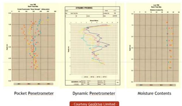
Above we reproduce the results from tests undertaken at the BRE research site at Chattenden. The characteristic bulge of root induced clay shrinkage is clearly visible. The rig penetrometer matches the profile obtained using the neutron probe at Aldenham. At shallow depth we see the influence of ground evaporation, and at around 2mtrs bGL is the root induced bulge, each diminishing with distance from the row of Poplars.
