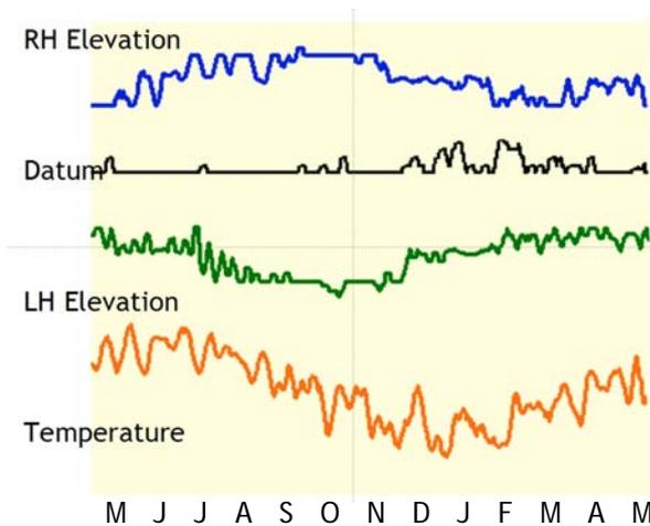
The black line is the datum, fixed to the LH side wall of the house. It is also being influenced by tree root activity, although less than the electrolevels fixed to the LH side wall of the extension, nearer to the trees.
