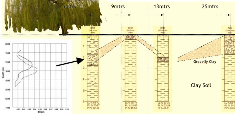
Oedometer, Disturbed –v– Undisturbed. BH 1
